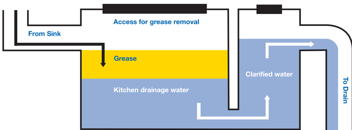
Diagram of an "under-the-sink" grease trap
